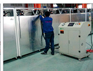
冷媒充注设备 Refrigerant filling equipment
